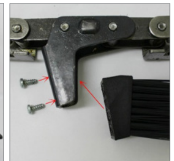
FIGURE 4: Short screws use lighter torque than standard brush blocks.
