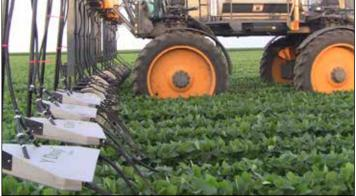
Figure 4. Coulter/Knife injection in 30" rows.
