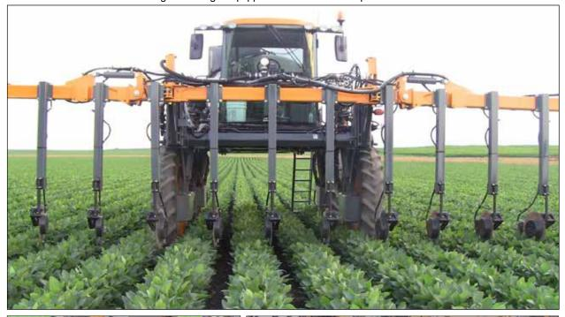
Figure 3. Hagie equipped with front mount liquid toolbar.
