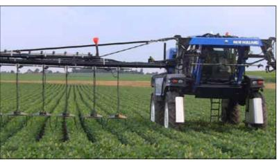
Figure 2. New Holland equipped with YDrop™.
