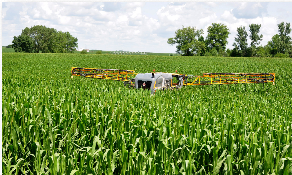
Greg Carson applies liquid nitrogen in a seed corn field in Cedar County on July 17, 2014. The N application is variable rated using a "Y" drop sprayer and an Ag Leader OptRx® crop sensor.
