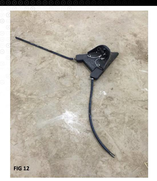
17. Attach riser tube assembly to 360 Y-DROP base unit using stainless steel wire lock pin, shown in FIG 13a & 13b. Repeat for every drop.
