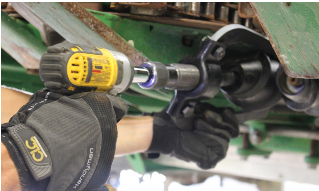
Extend hydraulic puller.
