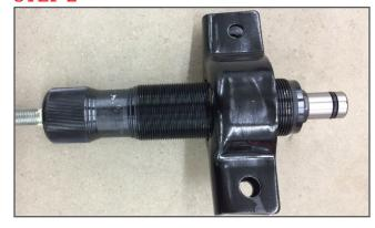
Slide the bracket over the threaded torque rod and onto the hydraulic ram. Place it over the threaded bushing.
