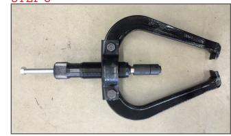
Install the extension shaft to protect the hydraulic ram, as shown. If you have factory/ OEM stalk rolls for John Deere 40 and 90 series corn head models, use the John Deere 40-90 extension shaft.
