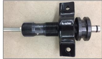
Thread the threaded bushing onto the hydraulic ram until it is in place with a few extra threads exposed on the side opposite of the threaded torque rod.
