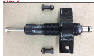
Before screwing the arms into the bracket and threaded bushing, notice the different sized holes on either side of the bracket. The head and nut of the bolt direction is opposite on each side, as shown. The smaller side hole is where you should secure the nut; the larger side hole is where the bolt head should sit.
