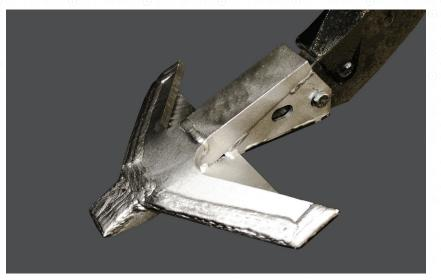
The streamlined shape and wide wings of the 360 BULLET ripper points generate a miniearthquake that fractures from point to point. That loosens the full soil profile for improved root penetration. Ultra-hardened material is welded to all wear surfaces for long life.
