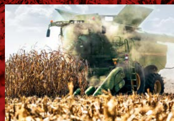
Cutting stalks precisely for pickup by row cleaners for a clear seedbed.
