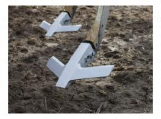
⊕ The streamlined shape and wide wings of the 360 BULLET ripper points generate a mini-earthquake that fractures from point to point, loosening the full soil profile for improved root penetration. CADI material provides the strength and wear resistance needed to withstand extreme conditions.
