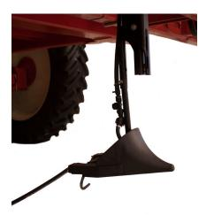
The aerodynamic base units allow 360 Y-DROP to move through the crop canopy. With the adjustable riser length, you can extend your sidedress season and take advantage of the yield gains that come from late season nitrogen application – even into V6 or V7.
