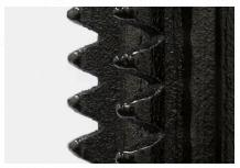
• Specially designed teeth for crimping the stalk.
