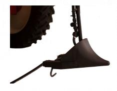
↔ The aerodynamic base units allow 360 Y-DROP to move through the crop canopy. With the adjustable riser length, you can extend your sidedress season and take advantage of the yield gains that come from late season nitrogen application – even into V6 or V7.
