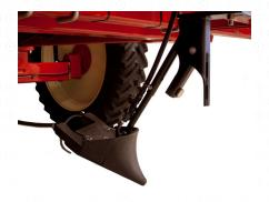
↔ The new breakaway riser offers the product protection. To protect the 360 Y-DROP base from ground impact, the system includes a magnetic breakaway riser mount. If you hit a wash or rock and the base releases from the bar mount, then immediately snaps back into position.
