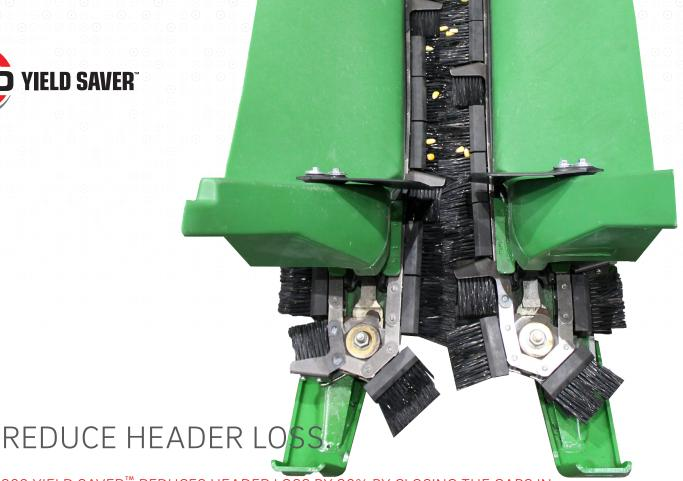
360 YIELD SAVER™ REDUCES HEADER LOSS BY 80% BY CLOSING THE GAPS IN TRADITIONAL DECK PLATES AND GATHERING CHAINS.
