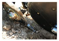
We've taken what we've learned from the 360 Y-DROP application placement system and adapted it to a system for the planter. The delivery tubes follow the coulter slot. Tension on the tubes keeps them in position over rough terrain and around contours.
