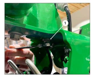
Using a 16mm socket, remove the M12 bolt ① second from the front of 360 BANDIT unit.
