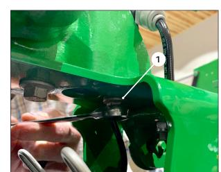
Using a 16mm socket, remove the M12 bolt ① second from the front of 360 BANDIT unit.
