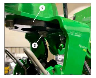
Place the saddle bracket support 2 on the underside of the 360 BANDIT unit and secure with the provided longer M12 bolt 3.
