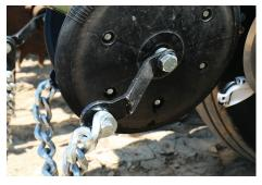
Simple mounting system. 360 DRAG CHAINs mount using the closing-wheel hub bolt. This mounting location provides added width and minimizes the overall bracket length.
