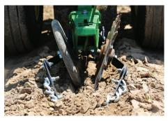
Wider coverage. 360 BANDIT places nitrogen in a band, three inches from the seed trench. The 360 DRAG CHAIN covers an eight-inch swath. That extra width ensures that the nitrogen slot is sealed and the seed trench is leveled.
