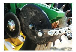
Each 360 DRAG CHAIN kit comes with a base and extension bracket. Use the base bracket for rubber and cast wheels. For spike closing wheels and other "paddle" types of wheels, use the extension bracket.
