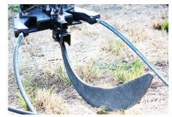
360 GLIDE uses a mechanical sensor rod to automatically maintain the ideal position of the 360 Y-DROP base. That keeps the delivery hoses in the right angle to deliver nitrogen directly to the base of the corn plant.
