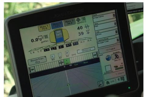
360 GLIDE plugs into your existing control system and you operate it just like you control your current system. No additional monitors. No elaborate configuration or settings.
