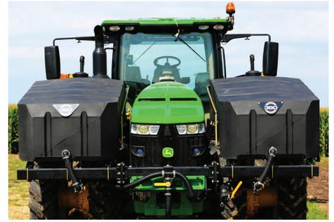
Narrow transport width. The tanks do not add to transport width. And, you still have access to the tractor's side panels for servicing.
