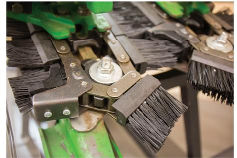
360 YIELD SAVER consists of a specialized gathering chain with crop lugs and replaceable brush blocks. Blocks quickly snap and screw into position and are easily replaced at the end of the harvest season.
