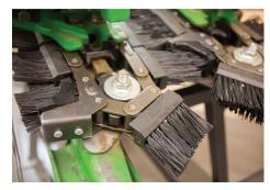
360 YIELD SAVER consists of a specialized gathering chain with crop lugs and replaceable brush blocks. Blocks quickly snap and screw into position and are easily replaced at the end of the harvest season.
