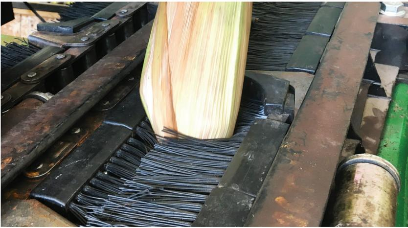
360 YIELD SAVERs reduce header loss with a combination of cushion and capture. Bristle blocks provide a softer landing for ears which means less shelling. Kernels that do come off the cob, are captured by long-lasting bristles and delivered to the cross auger.
