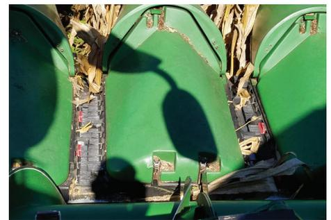
A corn head is a harsh environment, but 360 YIELD SAVER is built to withstand the abuse. Even when brushes show some wear, they are still delivering stray kernels and nubbins to the cross auger. Average brush block life is over 150 acres per row. Wear life of the chain is very similar to traditional gathering chains.
