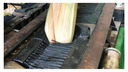
360 YIELD SAVERs reduce header loss with a combination of cushion and capture. Bristle blocks provide a softer landing for ears which means less shelling. Kernels that do come off the cob, are captured by long-lasting bristles and delivered to the cross auger.
