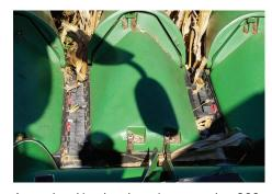
A corn head is a harsh environment, but 360 YIELD SAVER is built to withstand the abuse. Even when brushes show some wear, they are still delivering stray kernels and nubbins to the cross auger. Average brush block life is over 150 acres per row. Wear life of the chain is very similar to traditional gathering chains.
