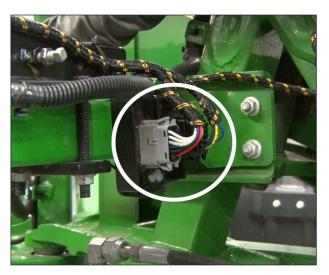
Plug the 12-pin plugs from the main harness into the combo board.
