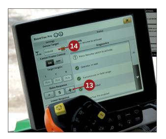
The raise response rate <sup>13</sup> can be adjusted according to your preference by clicking on the "-" or "+" buttons on either side of the numerical value in the "Raise Response" section. The higher the number, the faster the response.
