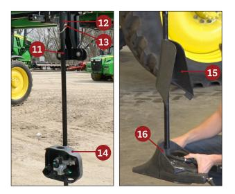
Install the risers  $\textcircled{1}{2}$  at each 360 GLIDE drop location by sliding the riser into the riser tube  $\textcircled{2}{2}$  on the three-magnet breakaway.
