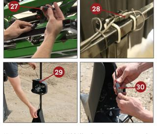
Using the drop harness (419312), plug the 4-pin receptacle connector into the previously routed boom harness Plug the 2-pin plug connector into the 2-pin receptacle connector on the three-magnet breakaway 8.
