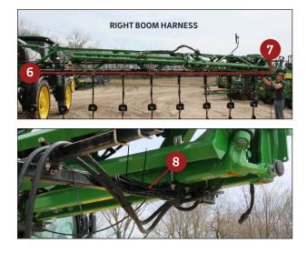
NOTE: The main extension harness has left, center and right specific connections. Ensure that each respective connection is routed to the correct side of the machine. Right and left are determined from the operators seat.
