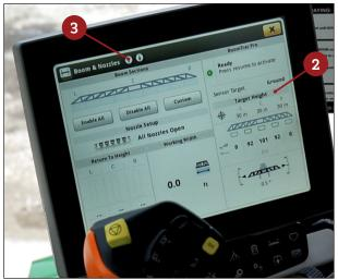
In the "Boom & Nozzles" window that opens, the boom height reading from the 360 GLIDE sensors is displayed to the right in the "Target Height" section **2**.
