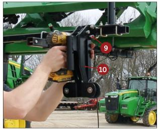
NOTE: If previously installed, 360 Y-DROP breakaways at the drop locations at center of the center section and the end of each primary boom MUST be removed and replaced with the new three-magnet breakaway.
