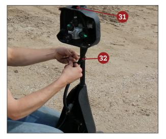
Reinstall the 360 Y-DROP hose, and if applicable, the 360 UNDERCOVER hose <sup>(1)</sup> by routing them from the OEM boom down through the 360 UNDERCOVER unit to the Y-DROP base unit.
