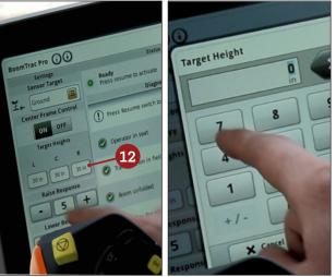
Click on the value under each sensor (L, C, & R) 1 to set the target height for each sensor location to match the reading from that sensor. E.g. if the actual sensor reading is a value of 75, the target height should be set to 75.
