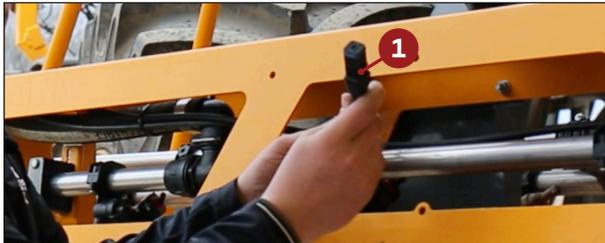
Unplug the five OEM Boom Height Sensors **1** located at the middle of the machine, each primary boom, and each secondary boom.
