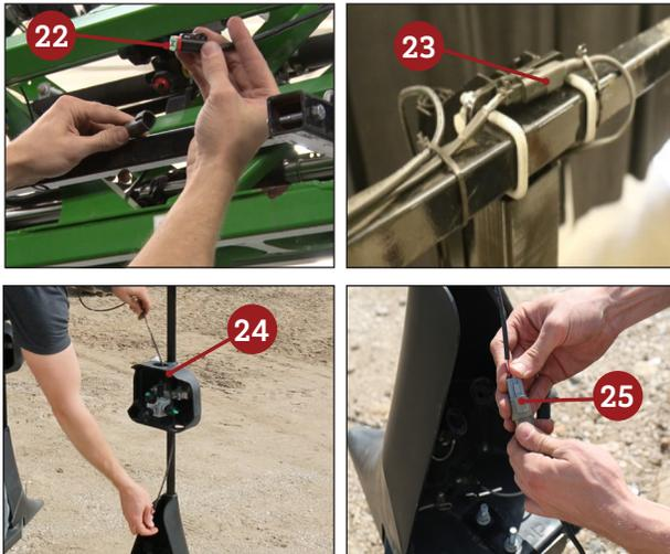
Using the drop harness (419312), plug the 4-pin receptacle connector into the previously routed boom harness **22**. Plug the 2-pin plug connector into the 2-pin receptacle connector on the three-magnet breakaway **23**.
