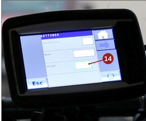
**NOTE: If using an AgLeader Integra display, set your measured height between 45-60 and match your target height to the measured height setting.**
