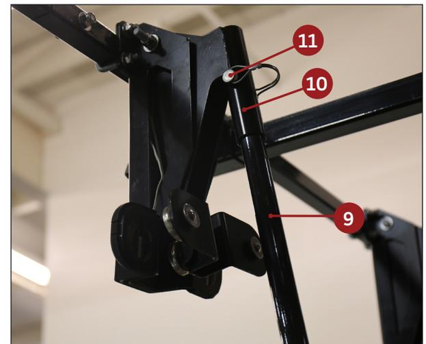
Install the risers **9** at each 360 GLIDE drop location by sliding the riser into the riser tube **10** on the three-magnet breakaway.
