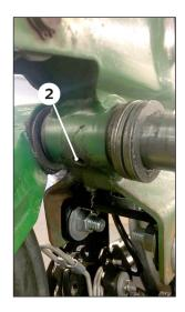
Using the hole on the bottom side of the shank ②, install the gauge wheel stop and spacer ③ using the 1-1/2" bolt and lock washer.
