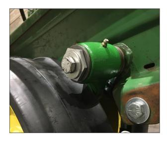
Reinstall the gauge wheel and adjust depth appropriately.
