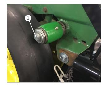
Remove one gauge wheel by loosening and removing the bolt 1 with a 3/4" socket.
