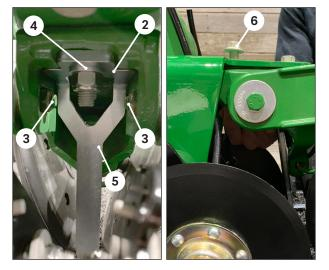
From the underside, maneuver the rock guard 2 around the two side bolts 3 and align the rock guard bracket with the hole in the BANDIT bracket and closing system 4. Ensure the guard extension 5 is to the rear.
