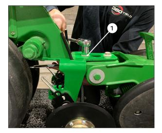
Using a 16mm socket and 19mm wrench, remove the front bolt 1 that secures the 360 BANDIT to the closing system. The bolt, washer and nut can be discarded.
