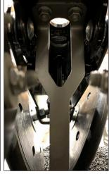
Orient the rock guard ③ so that the guard extension ④ is to the rear.
