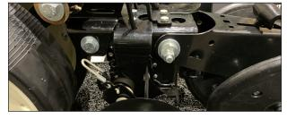
From the top, install the(2) provided 3/8" bolts **5** through the support strap, 360 BANDIT extension bracket and rock guard.
