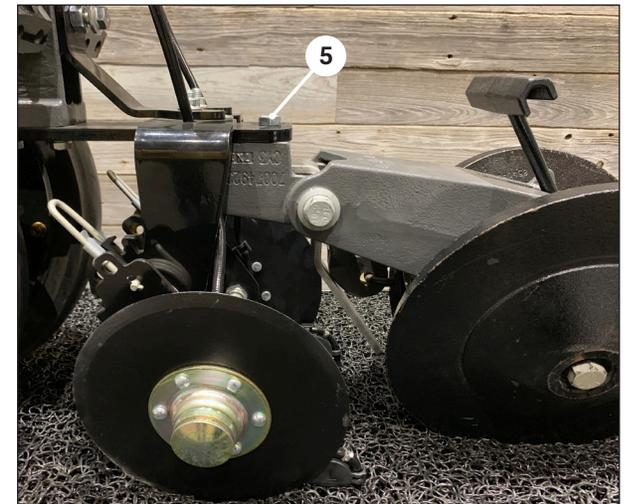
From the top, reinstall the bolt **5** through 360 BANDIT, closing system and rock guard.
