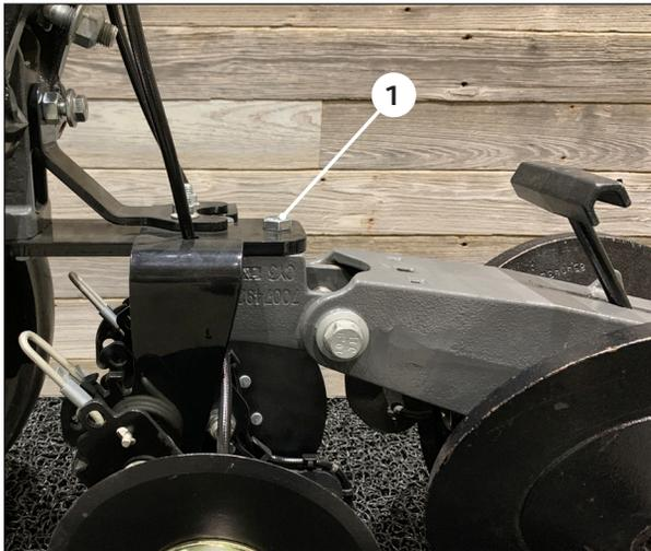
Using a 19mm socket and wrench, remove the rear bolt **1** that secures the 360 BANDIT to the closing system. The bolt and nut will be reused.
