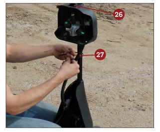
Reinstall the 360 Y-DROP hose, and if applicable, the 360 UNDERCOVER hose <sup>23</sup> by routing them from the OEM boom down through the 360 UNDERCOVER unit to the Y-DROP base unit.
