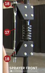
Install spacer blocks <sup>12</sup> by sandwiching riser above and below the spring. Ensure the nub on the block <sup>13</sup> goes into the indentation on the riser <sup>14</sup>.
