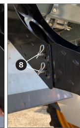
Install the drop extension 6 over the two %" tubes 7 on the mating bracket. Secure using the two 3/8" pins and hairpin clips 8.
