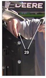
Feed the 6-pin plug end of the harness through the hole that top of the sensor guard assembly and plug it in to the rear of the factile sensor.
