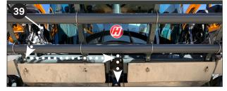
Attach the last 12-pin plug connector 60 to the gray receptacle on the controller 60.
