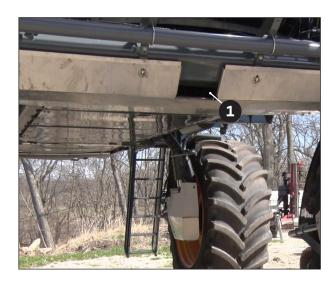
NOTE: If you have a high crop kit you need to replace the stainless shield with one from 360 Yield Center (Part #490319) that has a hole ① in it or you will need to cut the hole yourself to make room for the steering bracket.
