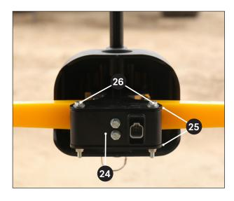
Place the wand/sensor assembly in between the upper and lower sensor brackets attached to the sensor guard assembly so that the top of the sensor is facing up and the wand is facing the front of the sensor guard assembly.
