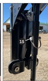
Mount steering breakaway 9 to the backside of the drop extension 6 using the 5/16" bolts, washers, and locknuts.
