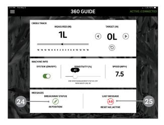
If the steering sensor has been pushed back enough to disconnect the magnet connection at the breakaway there will be an alert in the "BREAKAWAY STATUS" section of the operation page. When the breakaway re-engages, the alert will go away.
