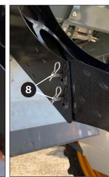
Install the drop extension 6 over the two %" tubes 7 on the mating bracket. Secure using the two 3/8" pins and hairpin clips 8.
