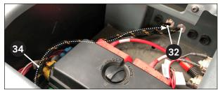
Starting from the front right dash panel, feed the two 4-pin connectors from harness 490232 labeled CAB A and CAB B from the front right dash panel up through the back right dash panel Leach connector will feed through one of the open access holes 2.
