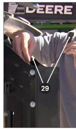
Feed the 6-pin plug end of the harness through the hole that the top of the sensor guard assembly and plug it in to the rear of the tactile sensor.
