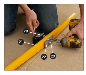
Using a 1/2" socket and wrench remove the hardware and plate on the steering sensor **20**.
