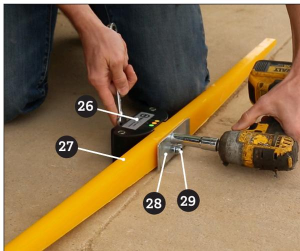
Using a 1/2" socket and wrench remove the hardware and plate on the steering sensor **26**.
