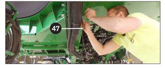
Connect the gray 12 pin connector on the harness to the gray port on the combo board 45. Use the extra black plug to fill the black port on the combo board.
