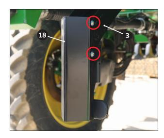
Mount steering breakaway to the backside of the drop extension using the 5/16" bolts, washers, and locknuts.
