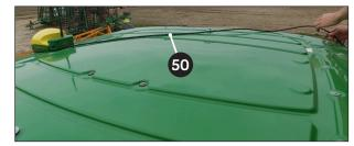
Plug in the 12 pin plugconnector into the GPS port embedded into the front of the cab, just below the GPS globe and bracket 49. Secure the harness on the back of the GPS StarFire mount with a ziptie, keepin g it on the outside and bottom.
