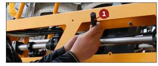
Unplug the five OEM Boom Height Sensors 1 located at the middle of the machine, each primary boom, and each secondary boom.
