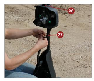
Reinstall the 360 Y-DROP hose, and if applicable, the 360 UNDERCOVER hose by routing them from the OEM boom down through the 360 UNDERCOVER unit to the Y-DROP base unit.
