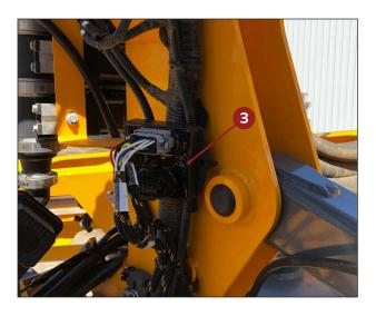
Plug the two 12-pin plugs from the main harness into the combo board 3. Place combo board in a safe location.
