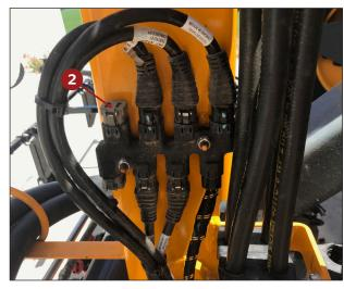
Plug the 12" harness adapter (419310) into the 4-pin receptacle connection of the main harness (419311).
