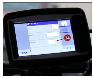
AGLEADER INTEGRA DISPLAYS ONLY: Set your measured height between 45-60 and match your target height to the measured height setting.
