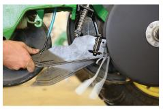
The spring-loaded 360 WAVE blade moves up and over obstacles to prevent damage, lower down force demands and maintain depth.
