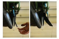
The 360 WAVE blade pivots - self aligning in the trench. That means it follows the trench on curves. A stop prevents the blade from pivoting over the seed trench on tight left turns.
