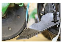
The liquid tube positions starter fertilizer 3/4" to the right of the seed trench and 3/4" below the seed. The hardened knife edge increases wear life.
