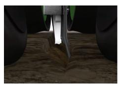
The 360 WAVE creates a "wave" of soil that rolls over the seed to simplify the job of the closing wheels.
