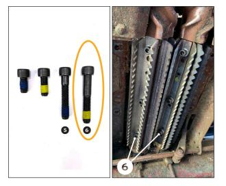
The longer M12 bolts will be used in the hole locations at the rear of the roll.
