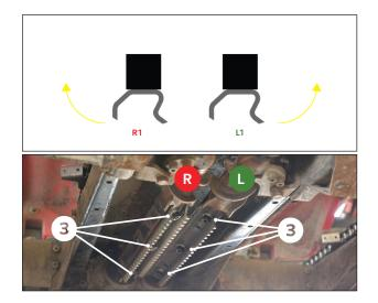
Using three of the <u>shorter</u> M12 bolts and lock washers from **hardware kit 450470** (3), install the **R1** plate on the **right roll**.
