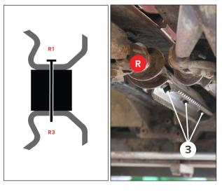
Using three of the shorter <u>through</u> bolts from **hardware kit 450471** (a) and three of the lock washers and flat washers from hardware kit 450470 install the R1 plate on the right roll.
