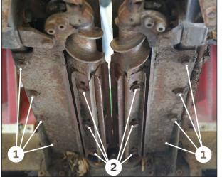
We have found the best way to install 360 CHAINROLL is by removing the residue knives and replacing the OEM roll knives with 360 CHAINROLL from the bottom side of the head.
