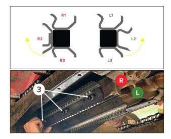
Using three of the <u>shorter</u> M12 bolts and lock washers from **hardware kit 450470** (3), install the **R3** plate on the **right roll**.
