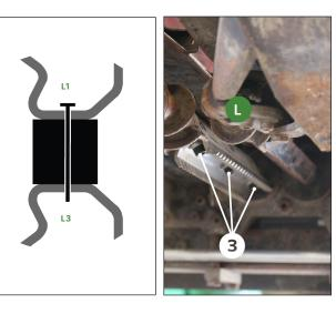
Using three of the shorter <u>through</u> bolts from **hardware kit 450471 (a)** and three of the lock washers and flat washers from **hardware kit 450470** install the L1 plate on the **left roll**.
