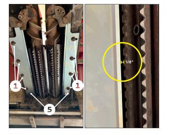
Using previously removed harware 1 install the 360 residue knives 6.
