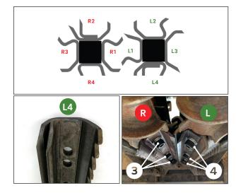
Using three of the <u>shorter</u> M12 bolts and lock washers from **hardware kit 450470 ()**, install the **R4** plate on the **right roll**.
