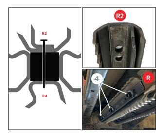
Using three of the longer <u>through</u> bolts from **hardware kit 450471** and three of the lock washers and flat washers from **hardware kit 450470** install the two **R2** plates on the **right roll**.
