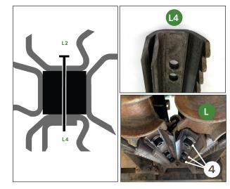
Using three of the longer <u>through</u> bolts from **hardware kit 450471** and three of the lock washers and flat washers from **hardware kit 450470** install the **L2** plate on the **left roll**.
