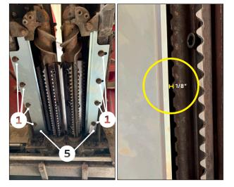
Using previously removed harware 1 install the 360 residue knives 6.
