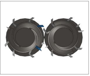
NOTE: Ensure cutting flutes are properly timed. As long as matching plates (R1 and L1, etc.) are adjacent to each other and the single cutting flute goes in between dual cutting flutes on the opposite roll, the rolls should be timed correctly.
