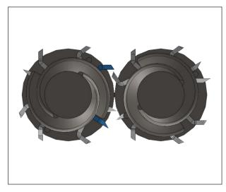
NOTE: Ensure cutting flutes are properly timed. As long as matching knives (R1 and L1, R2 and L2, etc) are adjacent to each other and the single cutting flute goes in between dual cutting flutes on the opposite roll, the rolls should be timed correctly.
