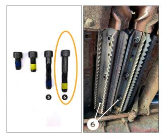
The longer M12 bolts will be used in the hole locations at the rear of the roll.
