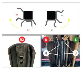
Using two of the <u>shorter</u> M12 bolts with <u>yellow loctite</u> and lock washers from <u>hardware kit 450640</u> (a), install the two R2 plates on the <u>right roll</u>. Bolts should be inserted at the appropriate locations at the front and middle of the roll.
