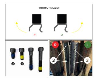
Using two of the <u>shorter</u> M12 bolts (**blue loctite**) and lock washers from **hardware kit 450640** (3), install the R1 plate on the <u>right roll</u>. Bolts should be inserted at the appropriate locations at the front and middle of the roll.
