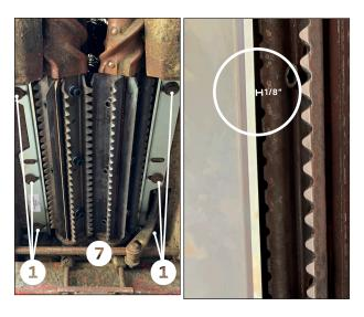
Using previously removed harware **1** install the 360 residue knives **7**.
