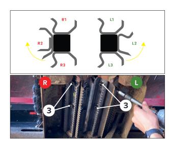
Using two of the <u>shorter</u> M12 bolts with **blue loctite** and lock washers from **hardware kit 450640** (3), install the R3 plate on the <u>right roll</u>. Bolts should be inserted at the appropriate locations at the front and middle of the roll.
