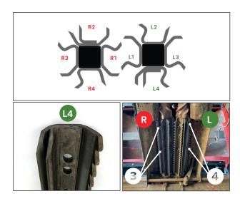
Using two of the <u>shorter</u> M12 bolts with **blue loctite** and lock washers from **hardware kit 450640** 3, install the **R4** plate on the <u>right roll</u>. Bolts should be inserted at the appropriate locations at the front and middle of the roll.
