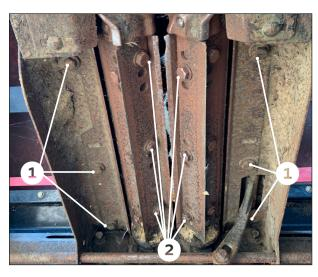
We have found the best way to install 360 CHAINROLL is by removing the residue knives and replacing the OEM roll knives with 360 CHAINROLL from the bottom side of the head.
