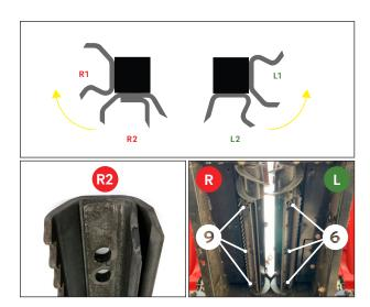
Using three of the <u>longer</u> M12 bolts and lock washers from **hardware kit 450420 9**, install the two **R2** plates on the **right roll**.
