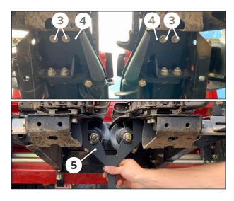
Remove the bolts 3 holding the covers 4 on the stalk roll bearings and set the covers aside. Retain all hardware.
