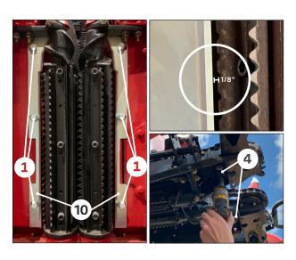
Using previously removed harware 1 install the 360 residue knives 10.
