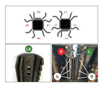
Using three of the <u>shorter</u> M12 bolts and lock washers from hardware kit 450420 ③, install the R4 plate on the right roll.
