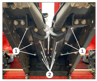
We have found the best way to install 360 CHAINROLL is by removing the residue knives and replacing the OEM roll knives with 360 CHAINROLL from the bottom side of the head.
