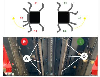
Using three of the <u>shorter</u> M12 bolts and lock washers from hardware kit 450420 **(3)**, install the R3 plate on the <u>right roll</u>.
