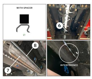
Using three of the <u>shorter</u> M12 bolts and lock washers from hardware kit 450420 **(3)**, install the L1 plate **(7)** and spacer **(3)** on the <u>left roll</u>. The spacer should be installed between the L1 plate and the shaft.
