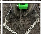
Using one new u-bolt and two new nylock nuts on each side, attach previous drag chain to the new chain bracket. Tighten u-bolts on chain and repeat for the other side.
