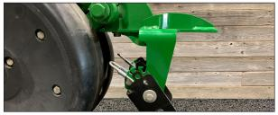
Using the two short M12 Bolts 4 attach the 360 BANDIT unit (long leg to the rear) to the row unit where the closing system casting was just removed.
