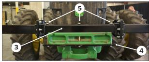
Using (12) 5/8" x 2-3/4" bolts, flat washers and nuts assemble three weight bracket beams 1 together. Install a flat washer on each side of joint.
