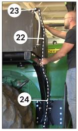
Install bottom 1-1/4" fitting into bulkhead towards the rear of the tank ②. Screw down to tighten and ensure port is faced to the rear.
