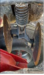
Case Early Riser 5 Series planters utilize offset closing disks, where one closingdisk is oriented slightly ahead of the second disk. The disk orientation of row units to the right side of planter center are mirrored to that of row units to theleft of planter center. Therefore, row units on the left side of your planter will require different brackets than row units on the right side. Install the left and right hand kits accordingly:
