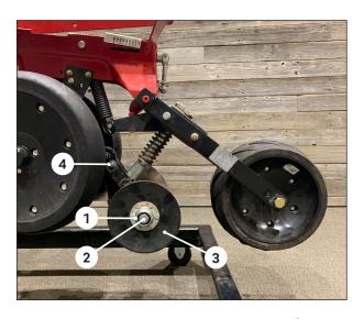
Using a chisel and hammer remove the dust caps **1** from each of the OEM disks. (NOTE: Picture shows dust caps already removed.)
