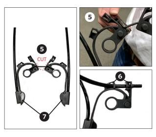
Using side-cutters, cut the two hose guides apart **5**.
