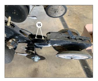
Using two remaining bolts and washers reinstall the closing system to the BANDIT unit <sup>19</sup>. Secure with nut.
