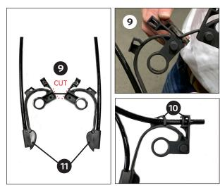
Using side-cutters, cut the two hose guides apart  $oldsymbol{9}$ .
