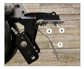
Insert one of the longer 1/2" bolts **6** through the rock guard **2** and then through the front hole on the closing system plate. Secure to the BANDIT unit.
