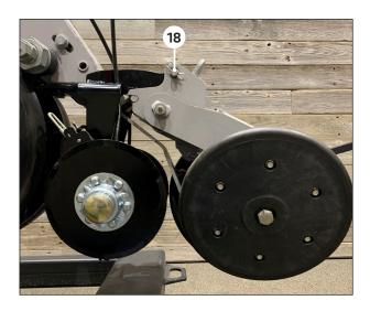
Slide the closing system into place, ensuring the pin hole lines up with the hole on the BANDIT unit.
