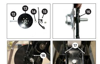
Insert 5/8" X 3" bolt through the disk 3. Insert bushing (large side first) and hose guide assembly (ear tab facing in).
