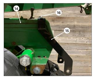
Using a 9/16" socket, remove the bolt from the top of the depth adjustment assembly 40 and discard.
