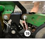
Attach the spring **10** to the spring hook **10** on the extension bracket.
