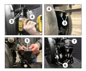
Using short M12 Bolts () install BANDIT extension bracket () (with BANDIT arm assembly installation holes to the back) using the closing system holes.
