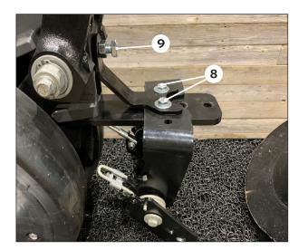
Align BANDIT arm assembly with the back horizontal holes on the extension arm. Align the support strap holes with the holes on the BANDIT arm assembly.
