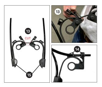
Using side-cutters, cut the two hose guides apart 13.
