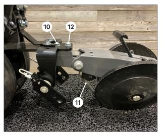
Using one of the long M12 Bolts and a nyloc nut, attach closing system to the second to last back hole in the BANDIT extension bracket <sup>10</sup>.
