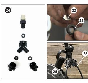
Install orifice plates  ${f a}$  in the rubber grommets  ${f a}$ .
