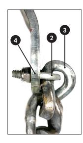
Using one u-bolt 2 on each side, attach drag chain 3 to chain bracket 4. Secure with nuts. Using 7/16" socket, tighten u-bolts on chain.
