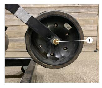
① Using a 15/16" socket and wrench, remove the 5/8" bolts on the press wheel.
