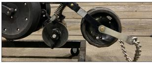
Insert the provided 5/8" bolt 1 through the chain bracket 4, left black bracket 5 on the row unit, press wheel 6, right black bracket bracket 7 on the row unit, and finally through the remaining chain bracket 8. Secure with nut 9.
