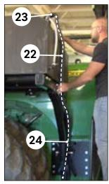
Install bottom 1-1/4" fitting into bulkhead towards the rear of the tank ②. Screw down to tighten and ensure port is faced to the rear.
