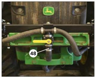
Install 2" flange/barb fitting onto end of 40' hose. Secure with hose clamp.
