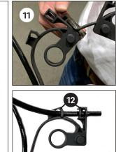
Using side-cutters, cut the two hose guides apart  $oldsymbol{0}$ .
