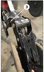
Attach the spring **1** from the OEM closing system to the hook **1** at the rear of the main BANDIT frame.
