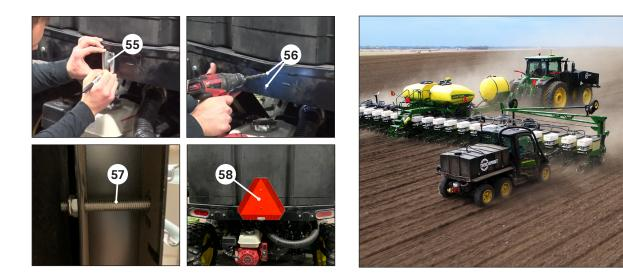
At the back of the SPRINT frame position the bracket <sup>(5)</sup> for the slow moving vehicle sign at the center of the frame and mark where the holes need to be drilled.
