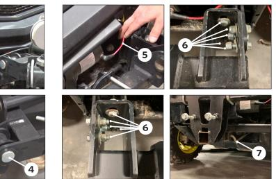
Disconnect the electrical connection to the winch under the hood of the gator. Once disconnected pull the electrical connection out of the front of the gator <sup>5</sup> and let it rest to the side.
