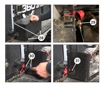
Remove the (3) thumb screws <sup>29</sup> holding the cover on the compressor box.
