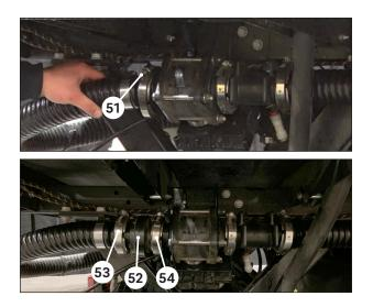
Using a 5/16" socket, remove the clamp <sup>(5)</sup> right before the on/off valve and remove the hose.
