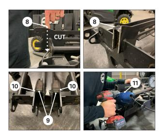
Modify the boom by using an angle grinder with a cut-off wheel to remove the existing winch cable bracket by cutting it at the cross brace <sup>(8)</sup>.
