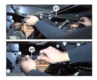
Route the tail light harness ④ along the SPRINT frame and connect it to the OEM connector ④.
