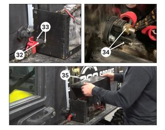
Insert the new switch  ${}^{\textcircled{32}}$  from the inside of the compressor box.
