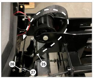
Route the winch strap under the roller, then over the top and back down towards the winch <sup>29</sup>. Be sure to keep the strap from twisting. Slide the pin <sup>20</sup> through the mount, strap and bracket on the other side and secure with hair pin clip <sup>20</sup>. The slack will be taken out of the strap at a later step.
