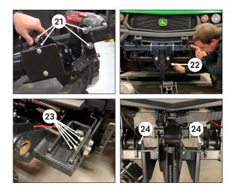
Attach the winch to the mount using the previous u-bolts, washers and nuts **1**. Tighten using a 9/16" socket.
