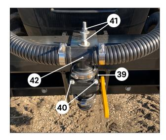
NOTE: Ensure there is a seal between every flange connection. And, for each hose installed during this process, each end of the hose should be secured to the fitting using the provided hose clamps.
