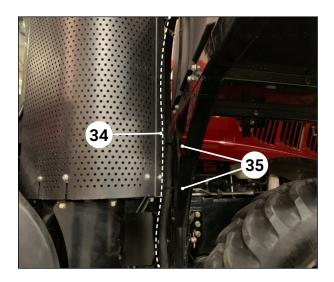
Route the 1-¼" EPDM rubber hose starting from where it is attached to the hose barb on the vent assembly continuing down along the rear support. Use zip ties to secure vent hose at multiple locations along the rear support. Trim the hose as you see fit.
