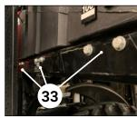
Using a forklift and fork extensions, lift the first tank off the shipping pallet. Ensure forks do not stick out past the tank so that they will not come in contact with the tractor.
