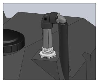
Install bottom 1-1/4" fitting ② into bulkhead towards the rear of the tank. Screw down to tighten and ensure port is oriented towards the rear.
